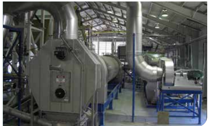
Commercial Airless Dryer with an evaporation rate of 2000 kg/hour (4400 lbs/hour)
